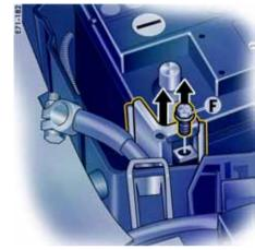
12.Unscrew screw **F** of the bracket. Remove bracket.
