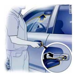
If you unlock the vehicle with the key at the door lock, only the driver's door is unlocked. In order to prevent the alarm system from being triggered, you must switch the ignition on within 15 seconds of opening the door.
