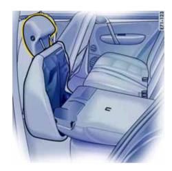
8. Insert headrest into the receiver in the seat cushion.
