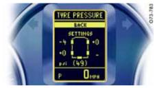
The spare wheel is not equipped with a wheel transmitter and is not monitored by Tire Pressure Monitoring. The tire pressure warning light on the speedometer flashes about 60 seconds and lights up thereafter permanently when the ENTER button is pressed. The value "\_" is displayed in the submenu TYRE PRESSURE (filling information) at the position of the spare wheel.
