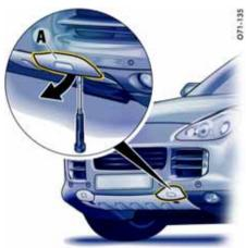
Screwing in front towing hook
