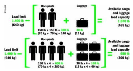
Example for determining the combined weight of occupants and cargo
