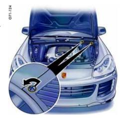
Cover of engine-compartment fuse box
