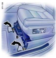
4. Fold sections of floor carpet forward. Unscrew both screws **B** of the seat mounting.
