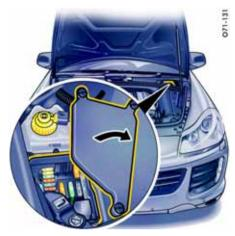
Fuse box in engine compartment
