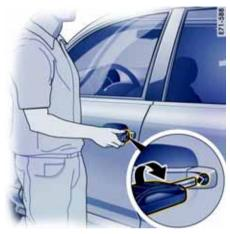
7. Lock the driver's door with the key in the door lock.
