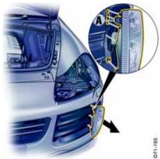
4. Press release tab **A** in direction of arrow again and push forward. Using your other hand, pull the bulb housing completely out of the front apron.
