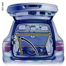
2. Unclip prop **B** and insert it into receiver **C** in the loadspace floor.
