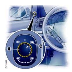
**A** - Control switch for door mirror adjustment **C** - Passenger mirror setting
