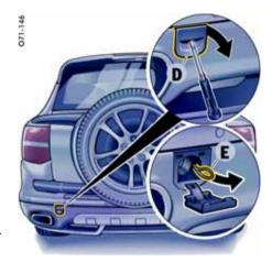
**D**-Towing lug cover (left) **E**-Emergency release cable
