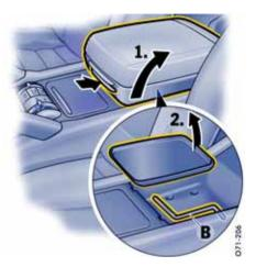
3. Remove key **B** from the lower storage tray (underneath the rubber mat) in the center console.
