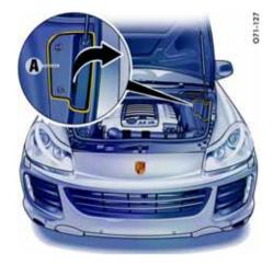
3. Remove cover **A** of the engine-compartment cover.
