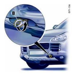
2. Screw in towing hook **B** as far as the stop (left-hand thread) and tighten hand-tight.
