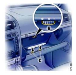
**B** - Thumb wheel for cooling the glove compartment **C** - Holder for pens
