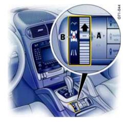
A - Rocker switch **B** - Low Range is engaged
