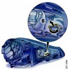
2. Turn bulb socket **B** counter-clockwise and remove.
