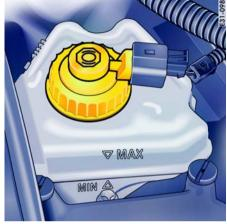
A slight decrease in the fluid level due to wear and automatic readjustment of the disc brakes is
