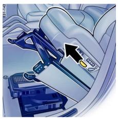
5. Tilt the seat all the way back. With the seat tilted back, use the fore-and-aft adjustment to move the seat forward again.
