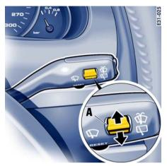
The rain sensor remains switched off if the wiper lever is already in position 1 when the ignition is switched on.
