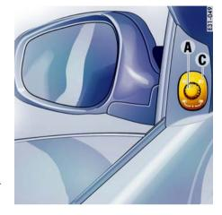
A - Control switch for door mirror adjustment
