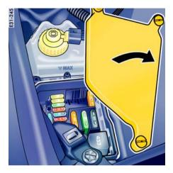
Fuse box in engine compartment
