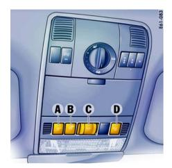
A, D - Switch for reading lights B - Button for dimming the comfort lighting C - Switch for interior light
