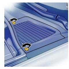
Cover of engine-compartment fuse box
