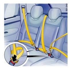
▶ Make sure that the belts and buckles fit correctly on the rear seat bench.
