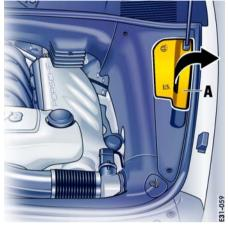
3. Remove cover of **A** the engine-compartment cover.
