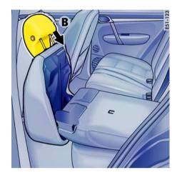
8. Insert headrest **B** into the receiver in the seat cushion (arrow).
