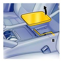
1. Remove key **B** from the lower storage tray (underneath the rubber mat) in the center console.
