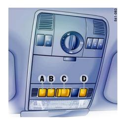
**A, D** - Switch for reading lights
