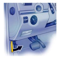
1. Pull release lever (arrow). Hood is unlocked.
