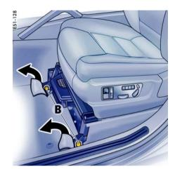
4. Fold sections of floor carpet forward. Unscrew both screws **B** of the seat mounting.
