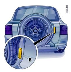
**B**-Button for unlocking the spare wheel bracket
