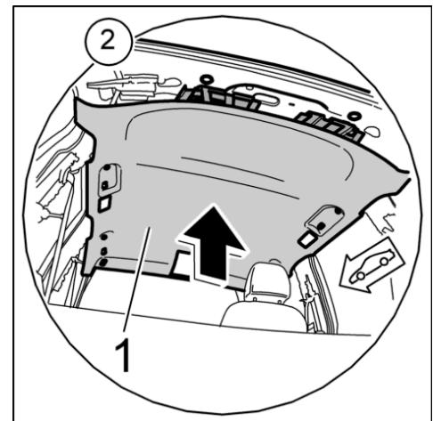
3. Clip fastening part for roof liner **-12-** into the bodyshell **-13-** at the back.
