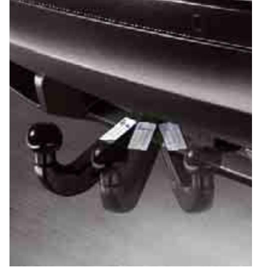
Towbar system with electrically deployable/retractable towball
