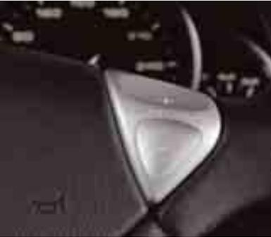
Tiptronic S gearshift control on steering wheel
