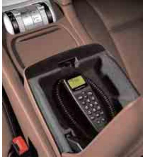
Telephone module for PCM with corded keypad handset
