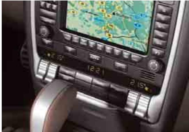
Air-conditioning control panel (cover open) below PCM
