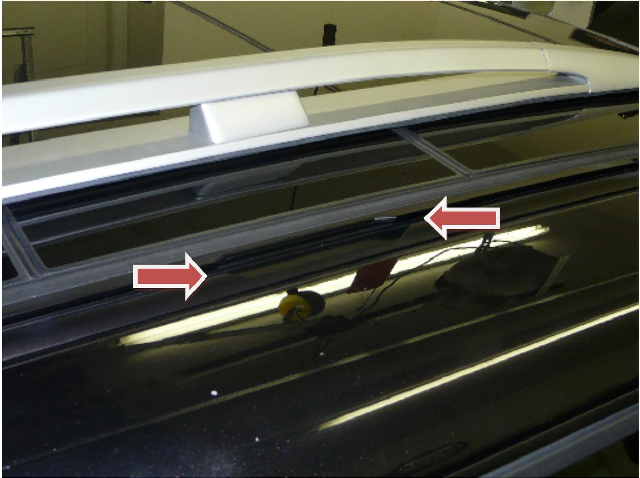
Start by inserting both “mL” adapters on each end and finally insert the middle adapter, please note that the allen bolt located on the side of the adapter must be facing the inside on the roof so these adapters can only install one way, again the allen head on the side must face on the inside.
