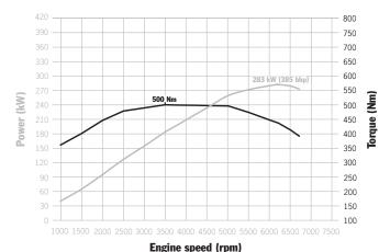
Cayenne S: 500 Nm at 3,500 rpm, 283 kW (385 bhp) at 6,200 rpm
