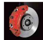
Cayenne Turbo: standard front brake with 368-mm disc
