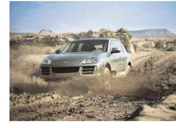
If that's not enough, the air suspension can be raised by another 30 mm to 271 mm (High Level II). At this setting, the new Cayenne models have an approach angle on gradients of 31.8° and a departure angle of 25.4°. The ramp breakover angle is 24.7°. The centre differential, part of the all-wheel drive system,
