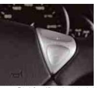
Tiptronic S gearshift control on steering wheel
