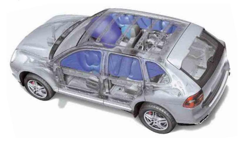
The driver and front passenger airbags use a gas generant based on an organic propellant. As a result, the airbags are lighter, more compact and easier to recycle.
