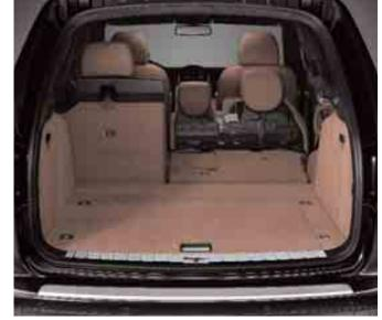
Loading option with rear seat backrest raised and loadspace cover retracted:
