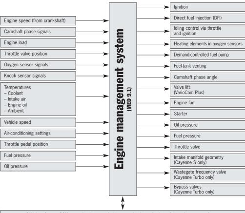
CAN interface to PSM control unit, transmission control unit, engine immobiliser, instrument cluster, air conditioning control unit, 'Sport' button, on-board diagnostics, etc.
