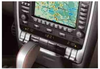
Air-conditioning control panel (cover open) below PCM
