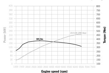
Cayenne: 385 Nm at 3,000 rpm, 213 kW (290 bhp) at 6,200 rpm
