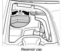
6. Carefully open the cap on the coolant reservoir. Unscrew the cap in an anti-clockwise direction.
