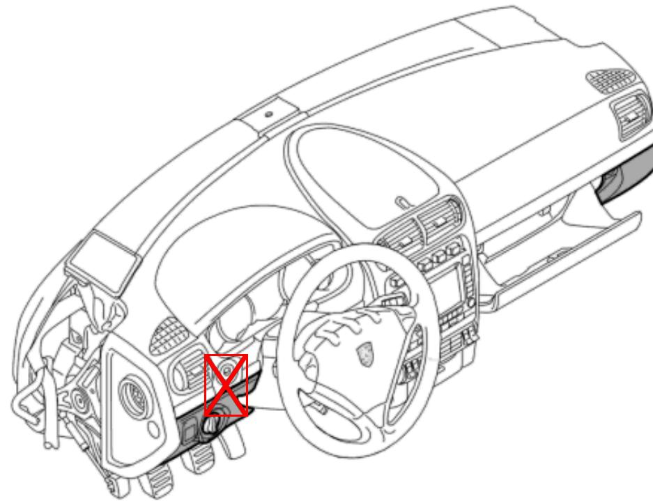
1. Insert the trim panel under the dashboard on the driver's side.
