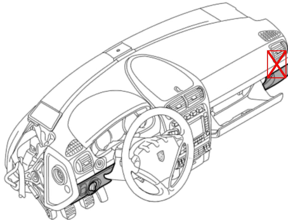
1. Remove dashboard moulding on passenger's side. → 705819 Removing and installing dashboard moulding on passenger's side - "Removing" section
