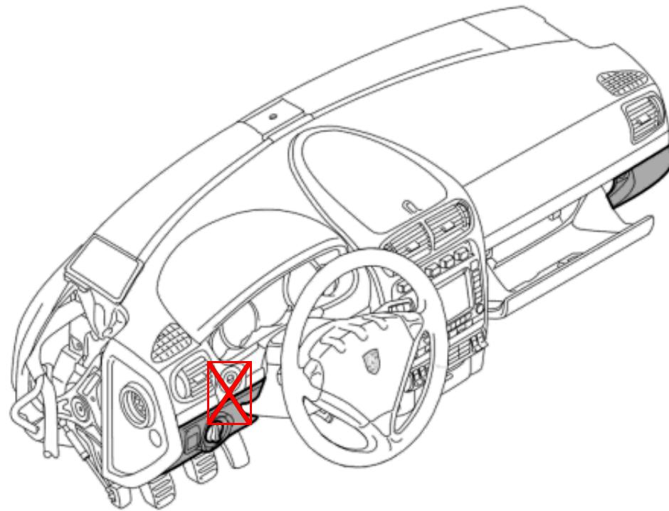
1. Remove dashboard moulding on driver's side. → 705819 Removing and installing dashboard moulding - "Removing" section
