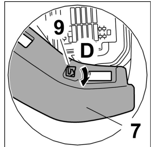
7. Disconnect the plug connection switch for the passenger's airbag.
