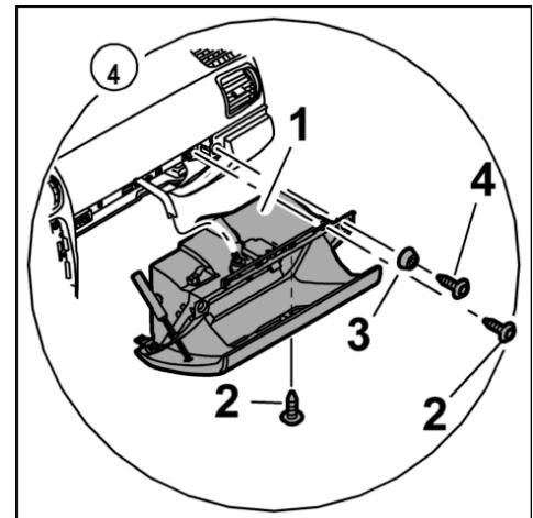
7. Install dashboard moulding on passenger's side. → 705819 Removing and installing dashboard moulding on passenger's side - "Installing" section
