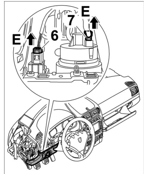
7. Unclip the bowden cable for the parking brake release.
