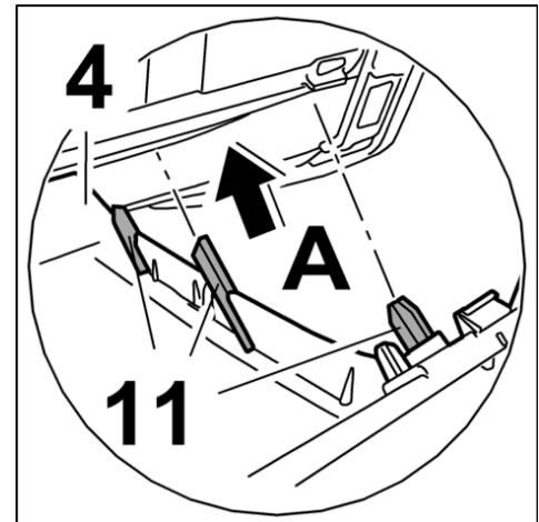
2. Clip in the bowden cable for the parking brake release.
