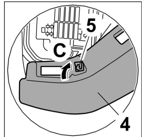
4.2. Swivel the trim under the dashboard on the driver's side **-4-** upwards **-arrow D-**.
