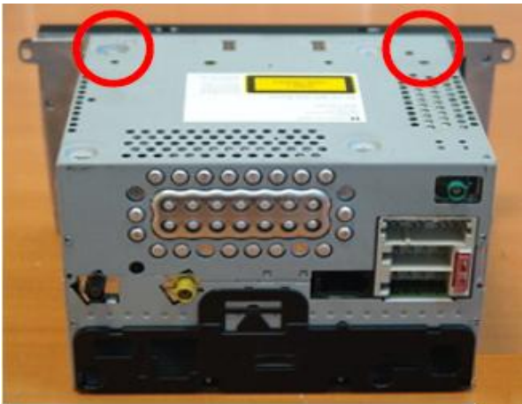
Step 1 : Take apart the screws marked with the tools.
