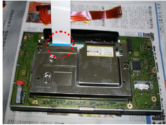
Step 6 : Connect the offered FFC cable to the connect where the brown FFC cable is connected.
