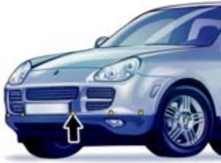
Front ultrasound sensors
