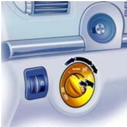
Light switch with driving light assistant
