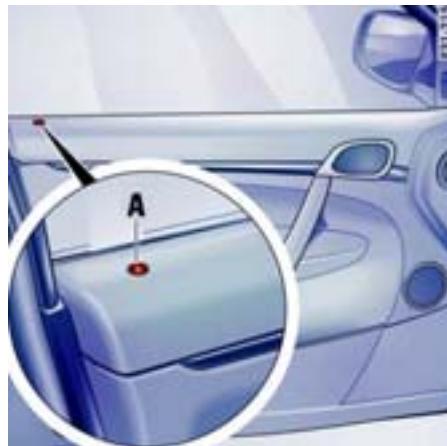
A - Light-emitting diode for alarm system
