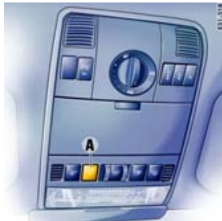
A - Button for dimming the comfort lighting
