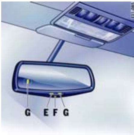
E - Light-emitting diodes (LED) F - Button for automatic anti-dazzle operation G - Light sensors
