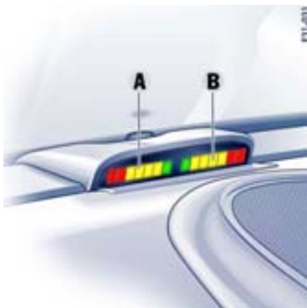
A - Front display – left monitoring area B - Front display – right monitoring area
