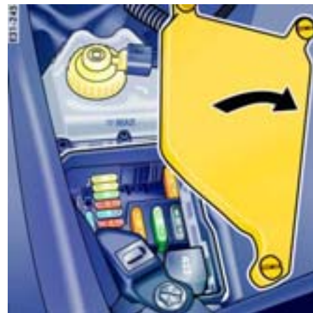
Fuse box in engine compartment
